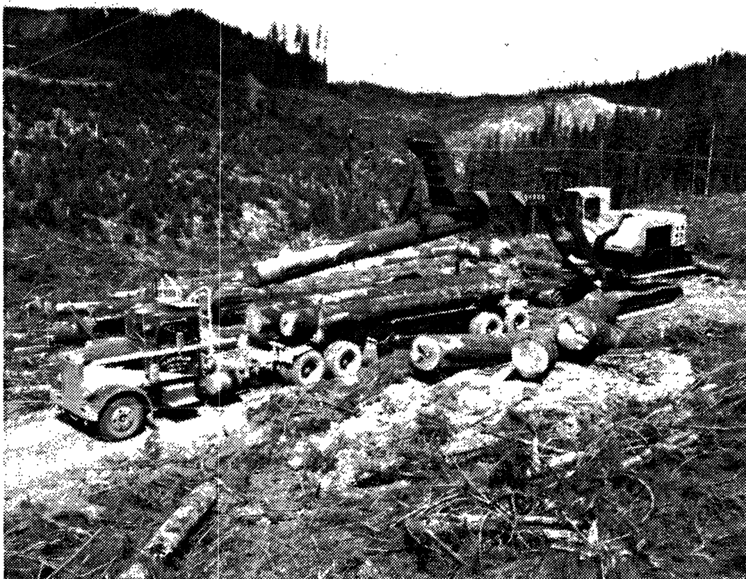
MODERN LOGGING OPERATION- Miller & Olson Logging Company operation in the Mill Creek area Southeast of Forks. One of the company trucks is being loaded with peelers by a new shovel. Reforested area is visible in the background.
